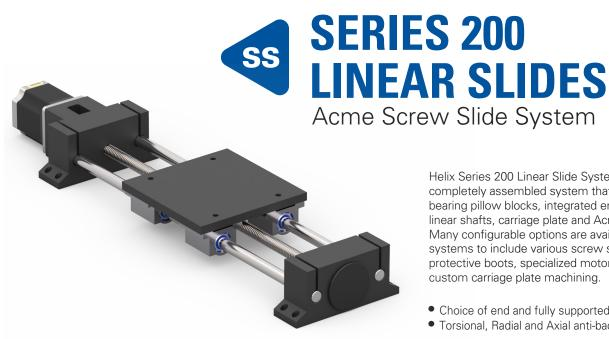
Helix Series 200 Linear Slide Systems come as a completely assembled system that includes: linear bearing pillow blocks, integrated end supports, HG linear shafts, carriage plate and Acme screw assembly. Many configurable options are available for these systems to include various screw styles and leads, protective boots, specialized motor mounts and custom carriage plate machining.
