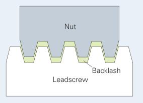
Imagine tightening a screw: you turn it a bit before you feel resistance, right? That initial turn where nothing happens is the backlash. In lead screw applications, backlash can be a concern because it can result in imprecise movements and reduced accuracy. Especially in applications where precision is crucial, such as CNC machines or 3D printers.
