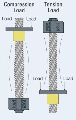
Thrust Load: A load parallel to and concentric with the axis of the screw.
